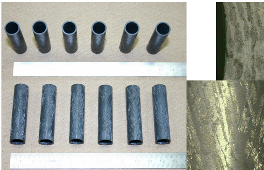
Fig. 2. Small diameter tubes of third generation pilot commercial grade (PG3) NITE SiC/SiC produced through the pseudo-isostatic hot-press technique.
